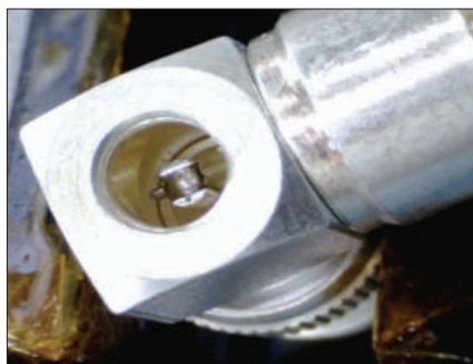
Fig. 4: Right angled BNC plug showing inner soldered.
