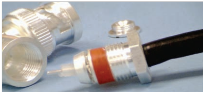
Fig. 3: A right angle plug and the coaxial cable with prepared end.
